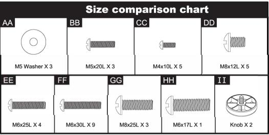
NOTE: Screw EE is **smaller** than Screw FF. Be advised that these are similar in size, please look carefully to ensure proper construction.
